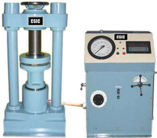
Figure 3.1 Compressive testing Machine
