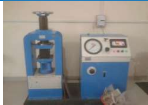
Figure 3 Compressive Strength test of geopolymer Concrete
