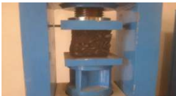
Figure 2 Compressive Strength test of geopolymer Concrete
