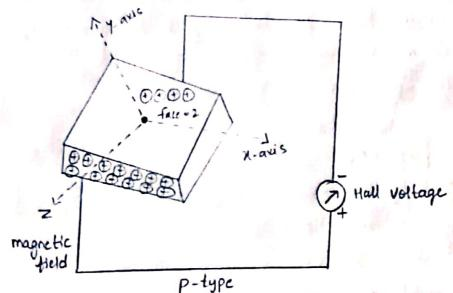
Now due to the magnetic field applied the holes move towards. The downward disection with velocity (v) and accumulates at the face (1). Therface a potential difference is established blw face (1) and (2) in the positive 4- direction.
