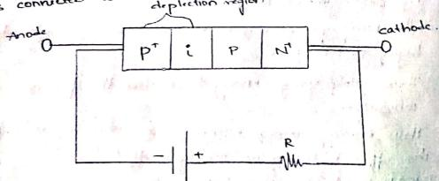
WORKING OF AVALANCHI PHOTO DIODE: > An incident light is passes through the Pt region on that time light should be interacting with charge carriers. => Later most of the Incident Light passes into intensic region
