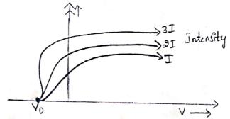
The above graph is photo electric current as a function of the potential difference of the two plates and different intensity of incident radiation.
